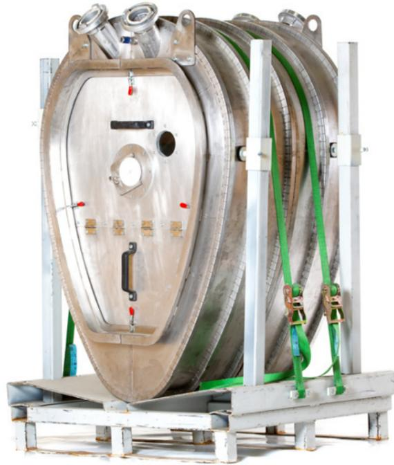
Most UV systems are equipped as standard with packer sets for the curing of liners up to DN 600. From DN 600, the requirements for the equipment change.
